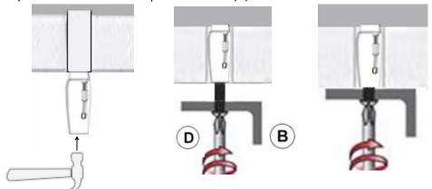
Step4: Thread screws(D) through the hanging units(B) holes, then tighten them into the tubes.
