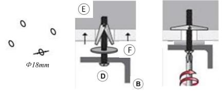
Step4: Tighten the screws.
