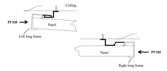
2. To avoid falling off, you must slide the panel left and right to make sure the two hooks have been completely put into the rear of the two long frames!
